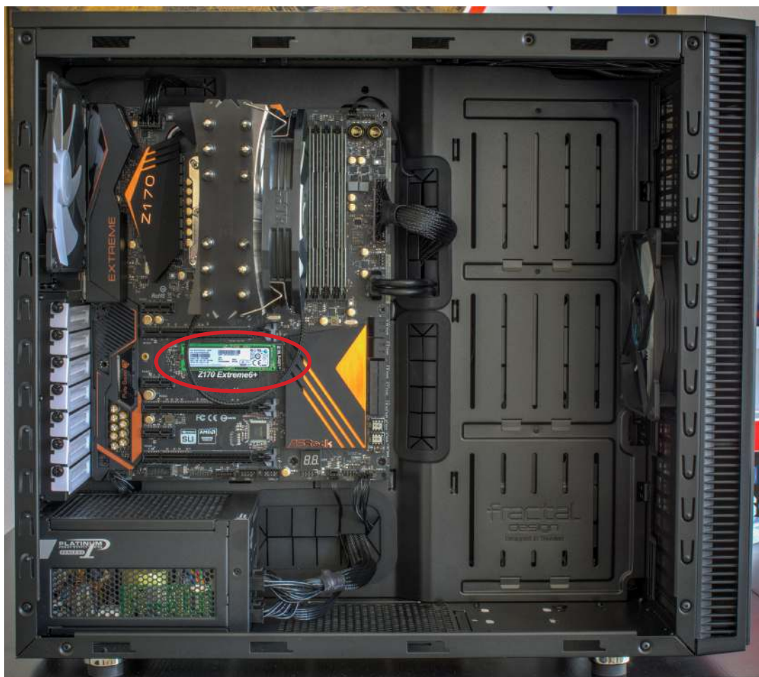
FIGURE 3: This image shows the incredibly small size of M.2 drives relative to a desktop case. That little stick is as thin as the PCB in a normal SSD.
